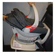
Remove infant carrier from base. The base can remain in the vehicle during visual inspection of carrier.
